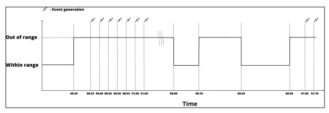
In the graph, it simulates an event condition, where there is a device within the range and later outside the ranges of acceptable values, causing the device to generate events.
